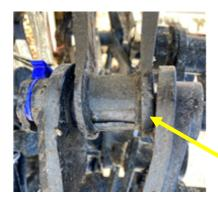
Failed Shaft Bearing
